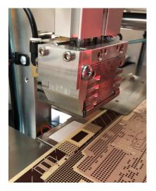
SmartWeld<sup>™</sup> is DIS's patented welding system. It consists of an upper and lower weld head. The complete weld cycle is controlled similar to a lamination press cycle. This allows rapid and precise heat control throughout a welding cycle giving more control to the process engineer.
